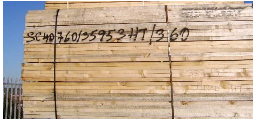
Photo: Coniferous wood from Russia intended for ISPM15 compliant wood packaging material manufacture and therefore marked as 'HT' heat-treated on the side of the pack – see section 2
