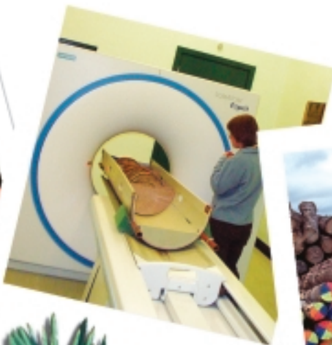
Using a medical CT scanner to measure the density of Sitka spruce discs
