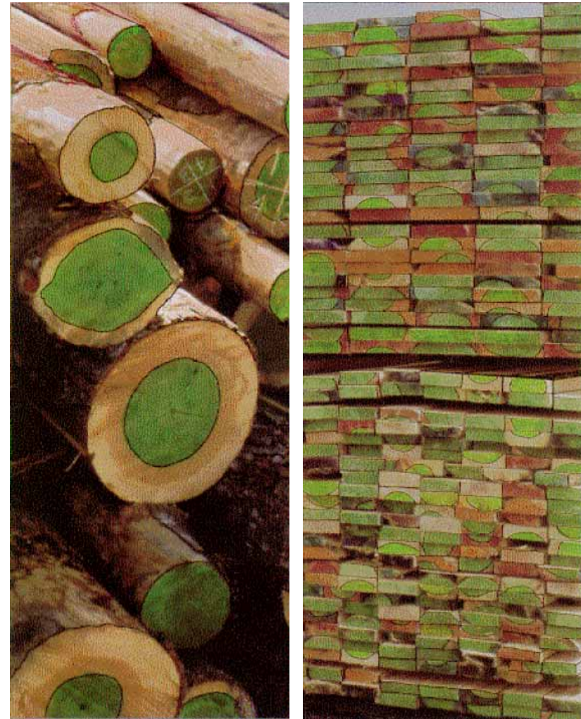
Fig. Juvenile wood (first 20 years of growth) marked on 50 year-old Douglas fir log and lumber ends
