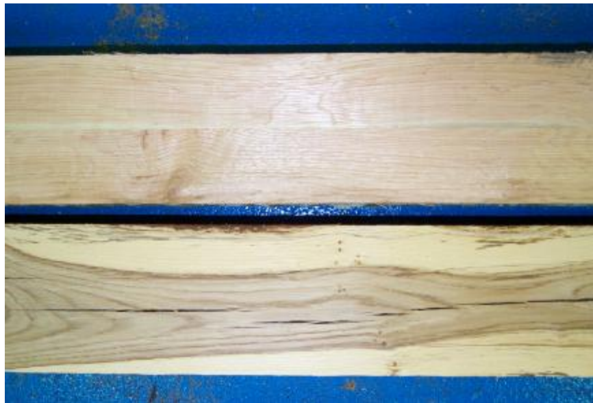
Figure 16. Air dried re-engineered oak beam above and comparable solid oak beam below
