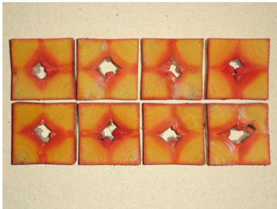
Figure 14. Preservative treated (after 3 months) re-engineered oak stems sprayed with an indicator to show treatment depth. Orange indicates preservative presence, yellow indicates preservative absence.
