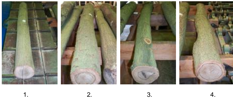
Figure 2. Stem straightness of oak logs categorised as per the Forestry Commission protocol
