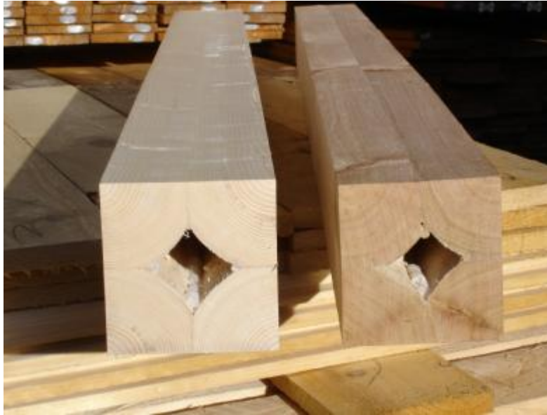
Figure 11. Re-engineered small diameter ash stem (left) and red oak stem (right)
