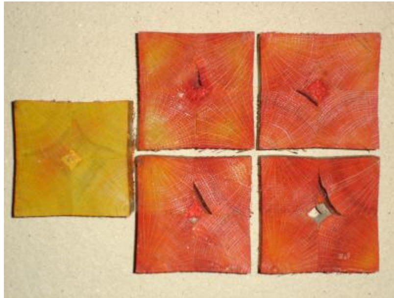
Figure 13. Preservative treated (within 2 weeks) re-engineered oak stems sprayed with an indicator to show treatment depth. Orange indicates preservative presence, yellow indicates preservative absence. The untreated control block is on the left.
