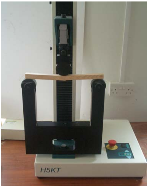
Fig. 3: Static bending rig with a small clear specimen in position.
