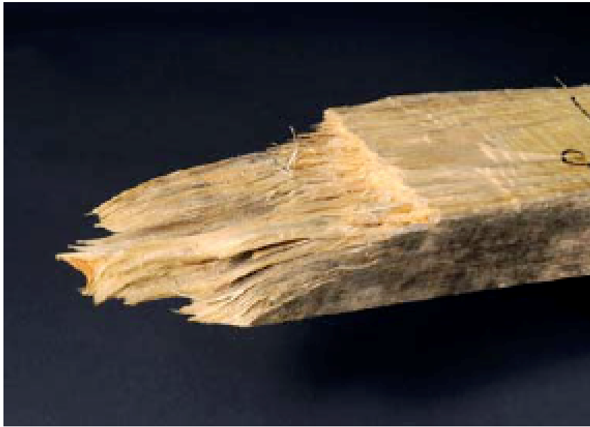
Simple Tension Failure
