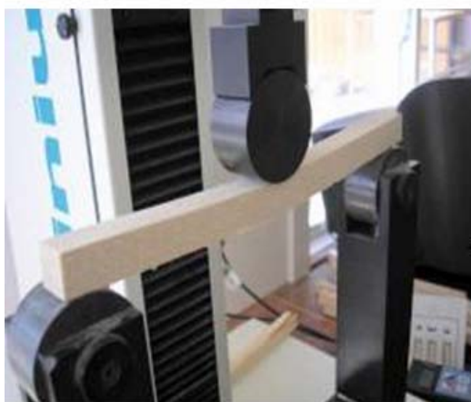
Mechanically testing for Strength & Stiffness
