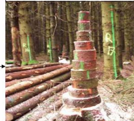
Measurement of branch sizes, and stem taper on felled tree
