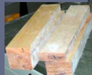
Kiln drying specimens (t = 25, 50 mm)
