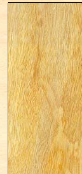
Oxidative staining of Framiré (Discolouration during kiln-drying)
